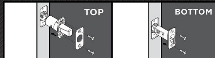
■ Install Top and Bottom Latches
